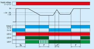
ND (neutral detection) – It occurs when the Neutral is not connected or it is disconnected during operation, or also when the voltage rises above 20 V (due to unbalance in the power grid). The maximum time delay is 350 ms for both the fault detection and the return of the ERWM to normal operation. For neutral detection, it is necessary to provide a bridge between terminals A and B; otherwise, the neutral will not be monitored.
