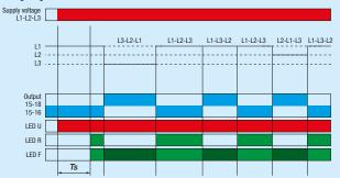
>Un (undervoltage) – It occurs after the rated tripping voltage (Un) (208 to 480 V) and the tripping undervoltage percentage (>Un) (-3 to -15%) are selected. The time delay is defined by the time scale (1 to 30 s) or disabled (OFF) acting in a maximum of 350 ms. The selected time delay is for both the fault detection and the return of the ERWM to normal operation.
