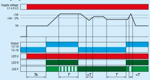
Asy (unbalance) – It occurs when the voltage of one, two or three of the phases vary, calculating the average value of the three phases and also the greatest voltage variation value by the average value. The worst voltage variation case is taken into account in the unbalance calculation. The time delay is defined by the time scale (1 to 30 s) or disabled (OFF) acting in a maximum of 350 ms. The selected time delay is for both the fault detection and the return of the ERWM to normal operation.
