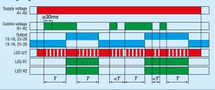
Da (symmetric flasher, start ON) – Applying the supply voltage, timing begins with times given by T1 (output ON) and T2 (output OFF). The cycle starts with the output relay energized. The times of full scale range T1 and T2 are the same. The total cycle is given by T = T1+T2. Interrupting the supply voltage with the output energized resets the time delay and de-energizes the output relay. This function requires the continuous application of supply voltage.
