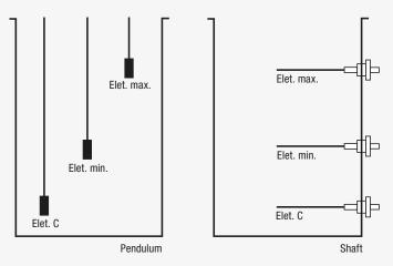
The shaft model (EHW) can be installed in the horizontal and vertical position
