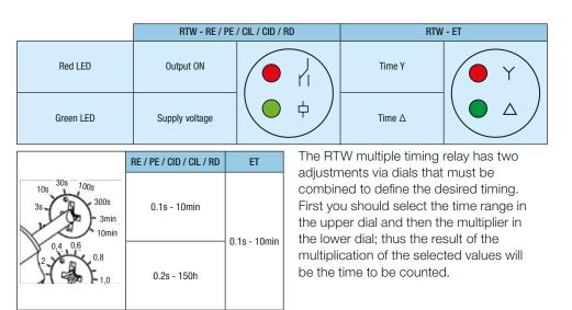
Notes: The RTW with multiple timing function must be reset at each new time range adjustment.
