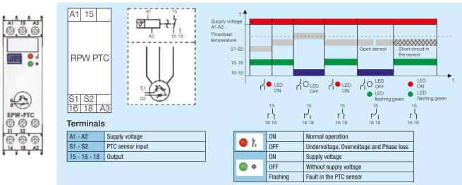
Notes: It is recommended the use of three PTC sensors in series, according to IEC 60947-8.
