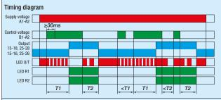
Dd (symmetric flasher, start OFF) – Applying the supply voltage, timing begins with times given by T1 (output 0N) and T2 (output OFF). The cycle starts with the output relay deenergized. The times of full scale range T1 and T2 are different. The total cycle is given by T = T1+T2. Interrupting the supply voltage with the output energized resets the time delay and de-energizes the output relay. This function requires the continuous application of supply voltage.
