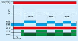
>Un (overvoltage) – It occurs after the rated tripping voltage (Un) (208 to 480 V) and the tripping overvoltage percentage (>Un) (3 to 15%) are selected. The time delay is defined by the time scale (1 to 30 s) or disabled (OFF) acting in a maximum of 350 ms. The selected time delay is for both the fault detection and the return of the ERWM to normal operation.
